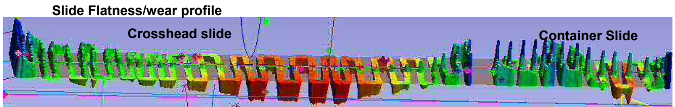
Figure 4. Deviations of scanned points from best-fit slide plane showing flatness and wear profile.
